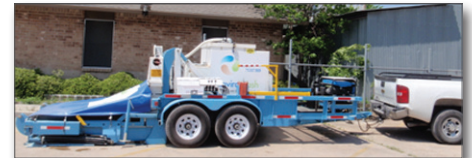
Figure 16. Washout container with a rain cover and onsite washwater treatment
