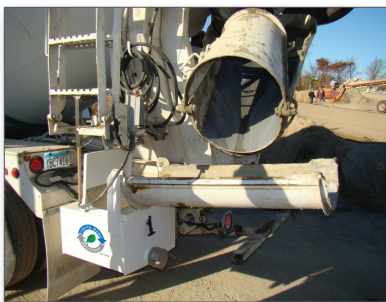
Figure 7. Chute washout box
